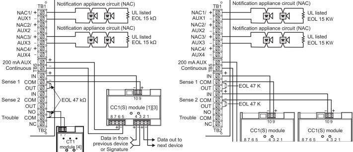
\*The Booster supports AC Power fail delay of three hours via its trouble contact when dip switch SW2-6 is on. All other troubles are reported to supervising module or panel without delay via Sense inputs.
